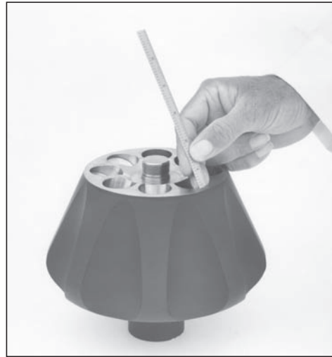
Figure 3. Measuring Distance from Cap to Rotor Tray
