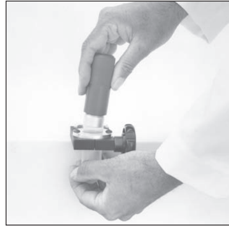
Figure 5. Pulling the Stem from the Tube
